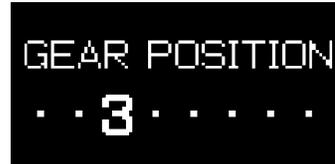
Third gear is in use and the shift lever is in D or the D8 range is selected.
