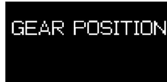
The shift lever is in a position other than D or M.
