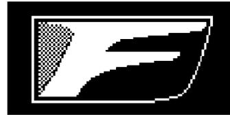
Display during 8-speed sport direct shift control (M position).
